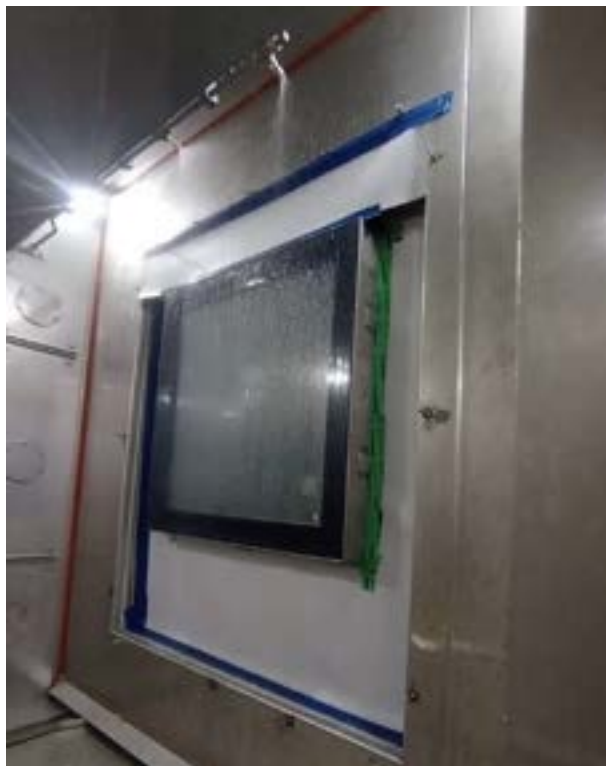
Fig. 5 Water tightness test in progress
