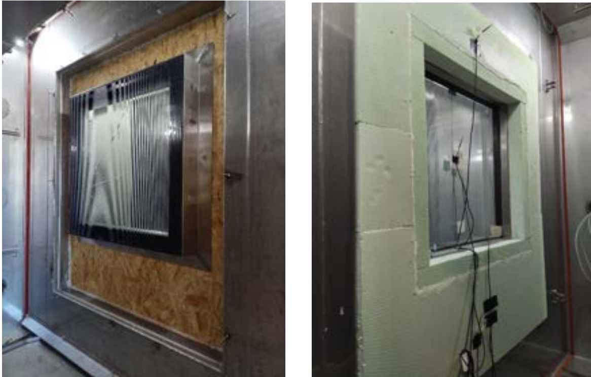
Fig. 7 Placement of the sample in the outdoor chamber (left), in the indoor chamber (right)
